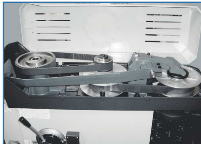
VS Variatore semplice Variable speed-drive unit
