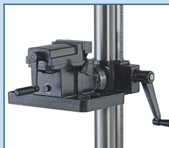
PGM: 350 x 250 mm Piano girevole morsa Tilting table with vice and rack
