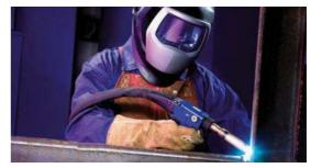
The screw-type torch necks can be replaced quickly. They are available as either straight or 45° angled versions. A special interface between the handle and the torch neck makes it possible to turn the necks up to 360°. All torches, both air and liquid-cooled for capacities of up to 400 A, are based on the tried-and-trusted "MB" torch neck design.
